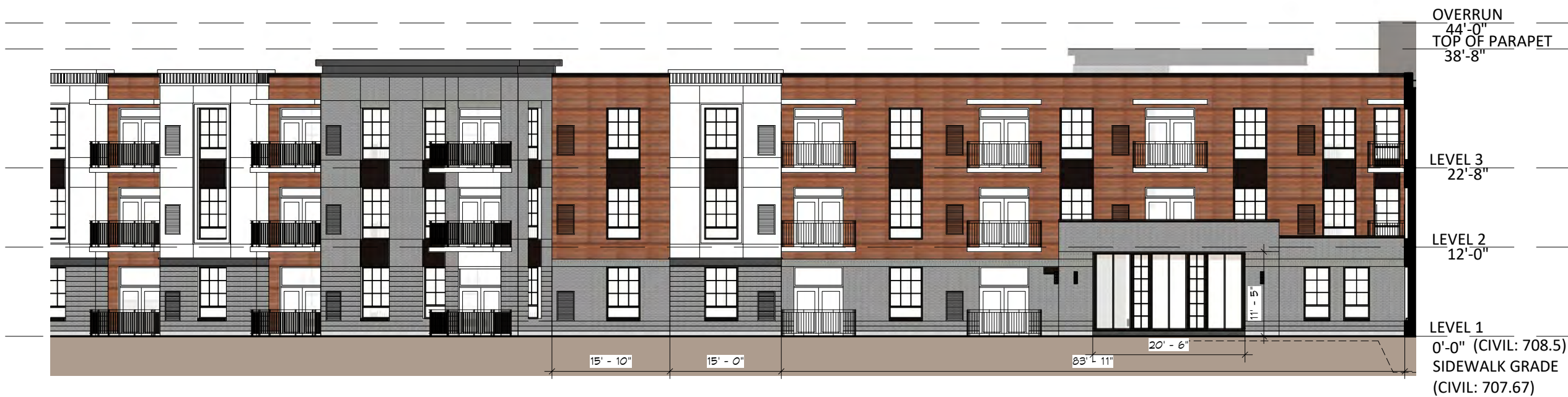
1 SOUTH - PARTIAL ELEVATION 1 A1-6 1/16" = 1'-0"
