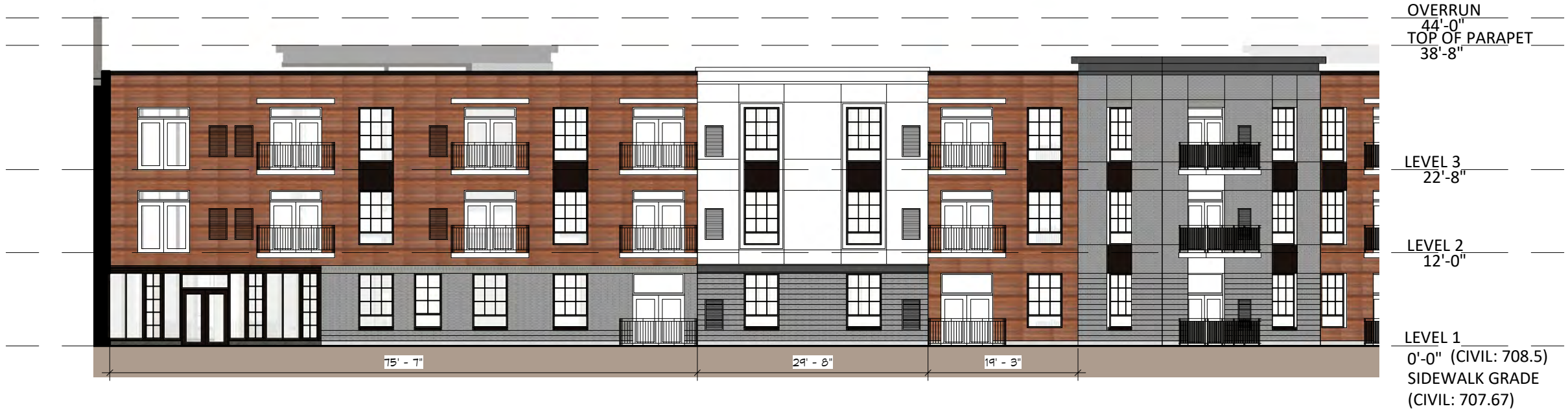
9 NORTH - PARTIAL ELEVATION 3 A1-6 1/16" = 1'-0"
