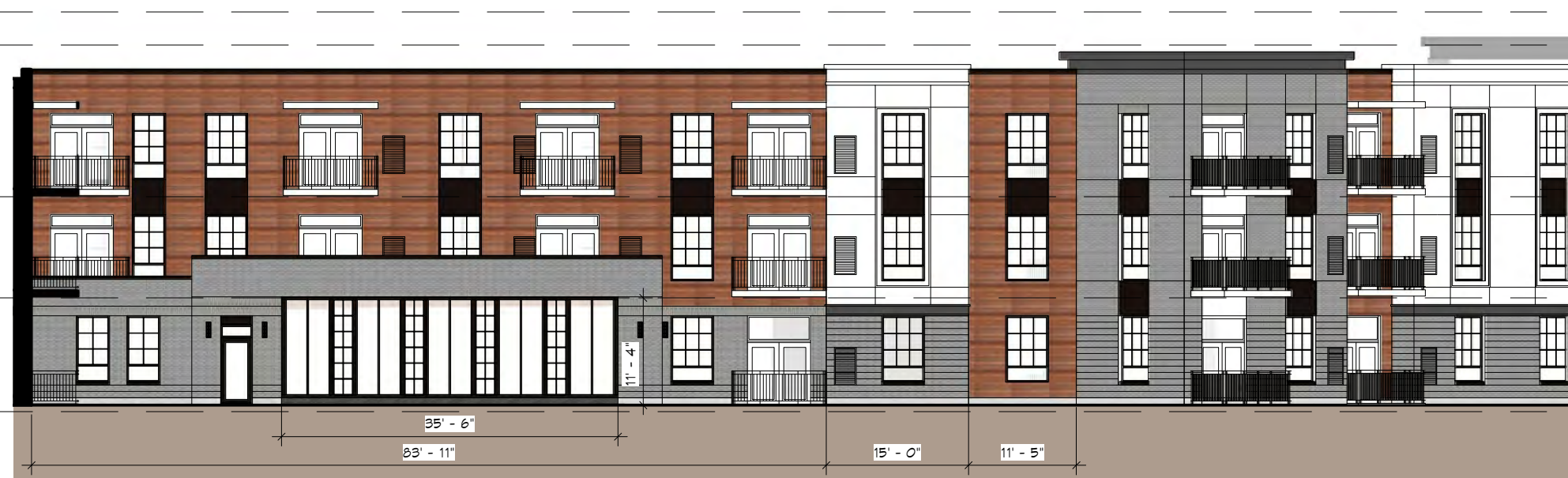
2 SOUTH - PARTIAL ELEVATION 2 A1-6 1/16" = 1'-0"
