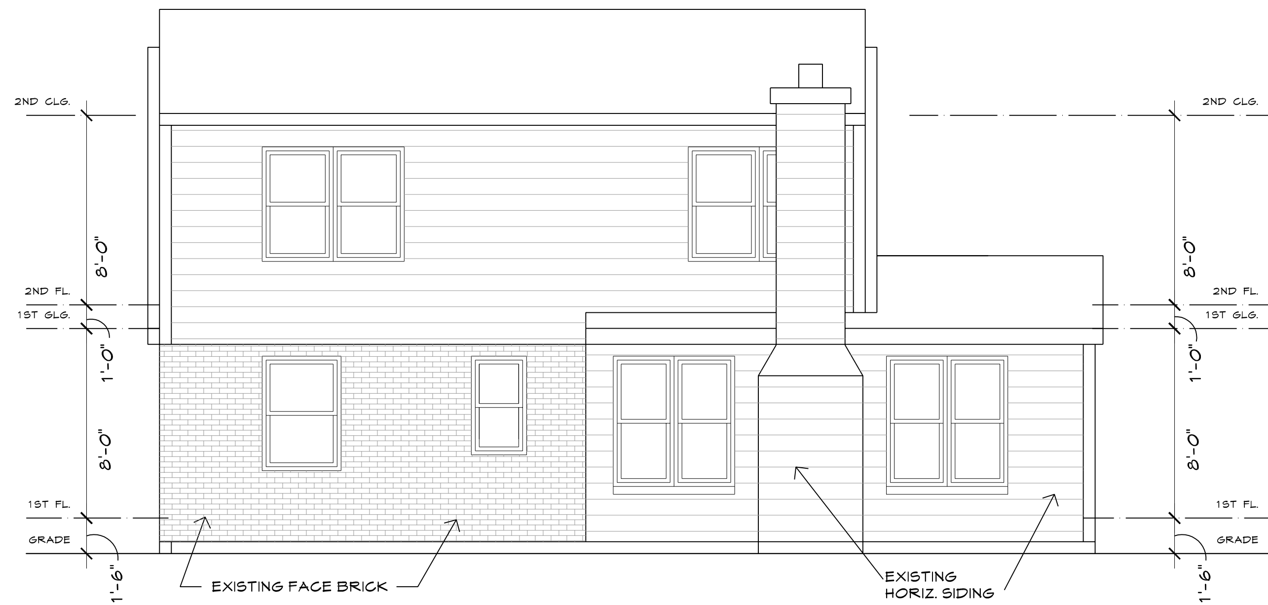
EAST ELEVATION (EXISTING)
