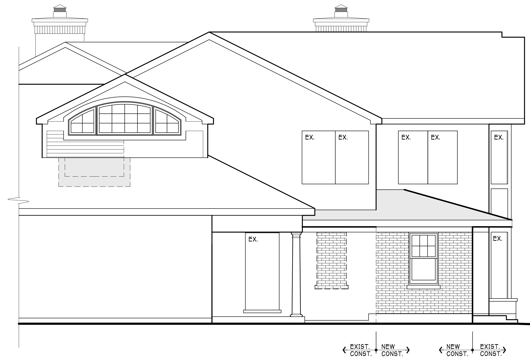
2 PARTIAL WEST ELEVATION A-3 1/4" = 1'-0"
