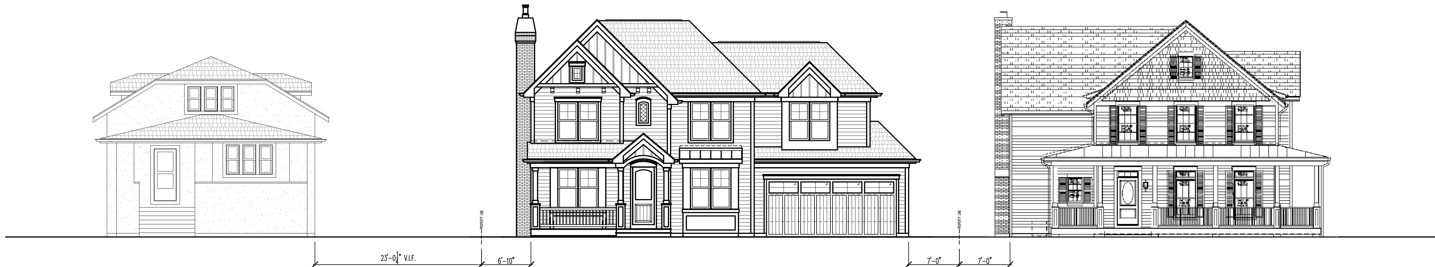
1C A201 EXISTING FRONT ELEVATION 1/8"=1'-0"
