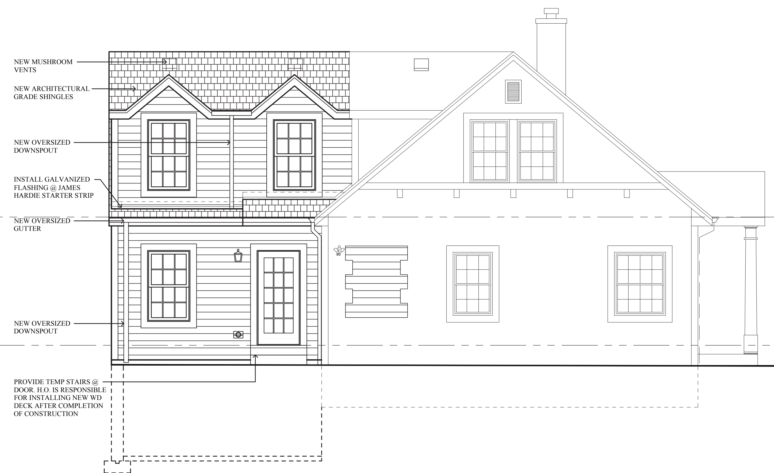
4 NEW NORTH ELEVATION 1/4"=1'
