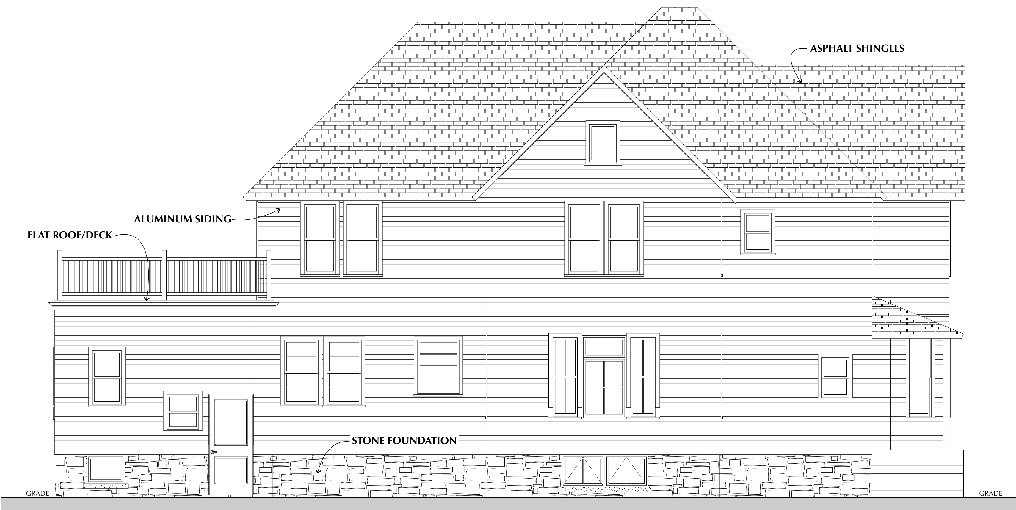
EXISTING LEFT ELEVATION
