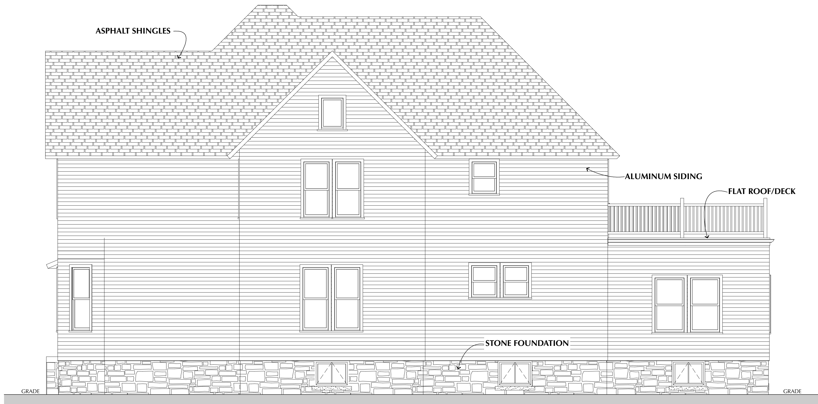
EXISTING RIGHT ELEVATION
