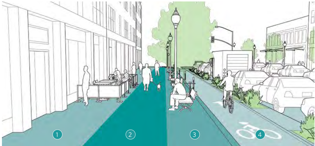
Figure 4.33 - Sidewalk Zone System
