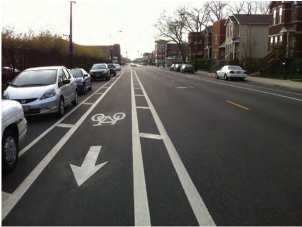
Figure 4.41 - Buffered Bike Lane
