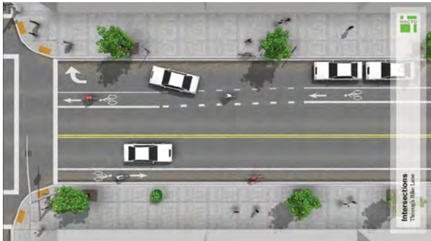
Figure 4.74 - Through Bike Lane Option B
