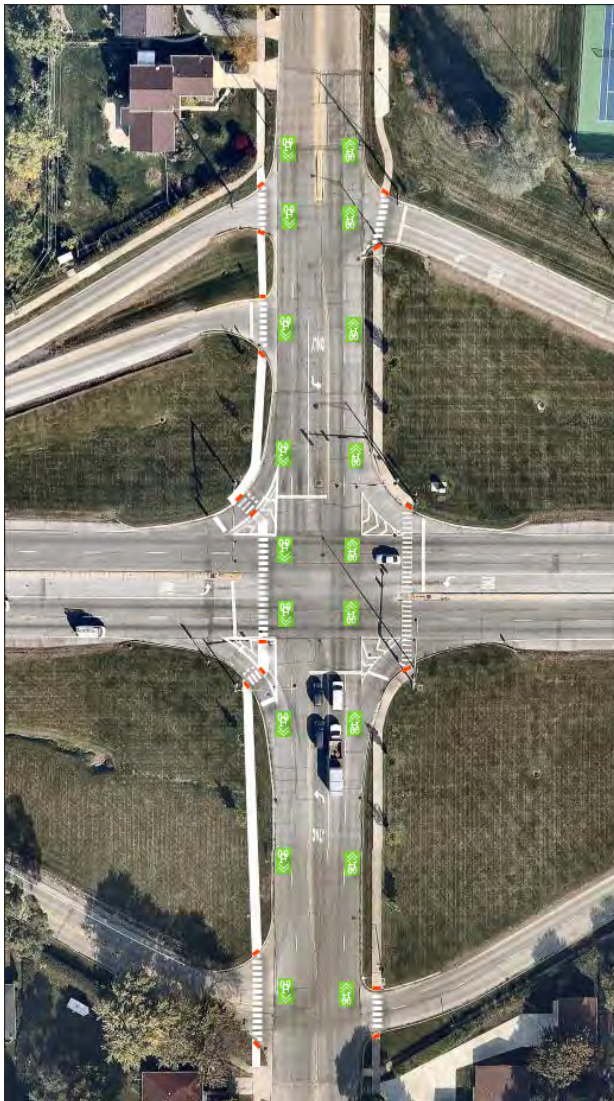
Figure 4.20 - Sharrows at Kennicott and Palatine
