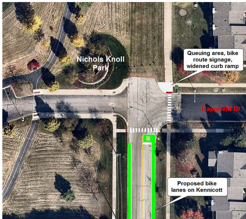
Figure 4.26 - Concept for transition at south end of Nichol Knoll Park Path
