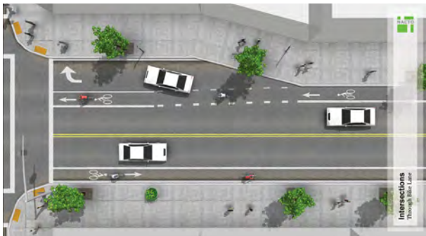
Figure 4.74 - Through Bike Lane Option B
