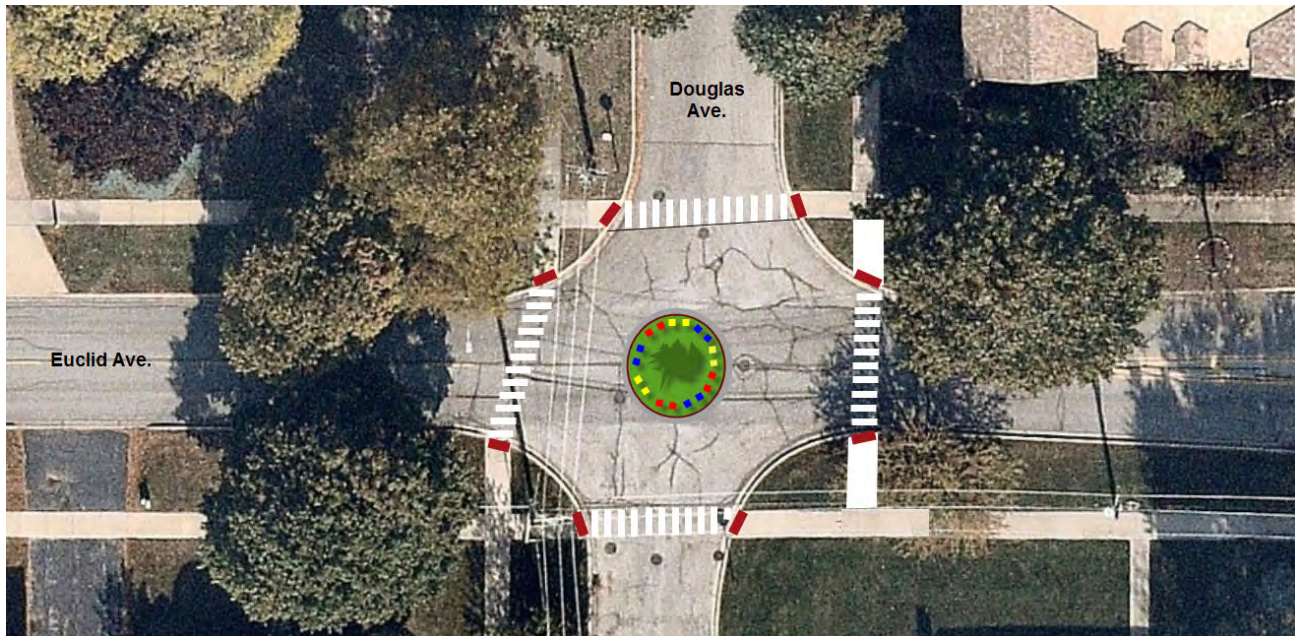
Figure 4.90 - Mini traffic circle at Euclid and Douglas
