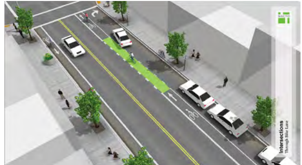
Figure 4.76 - Through Bike Lane Option D
