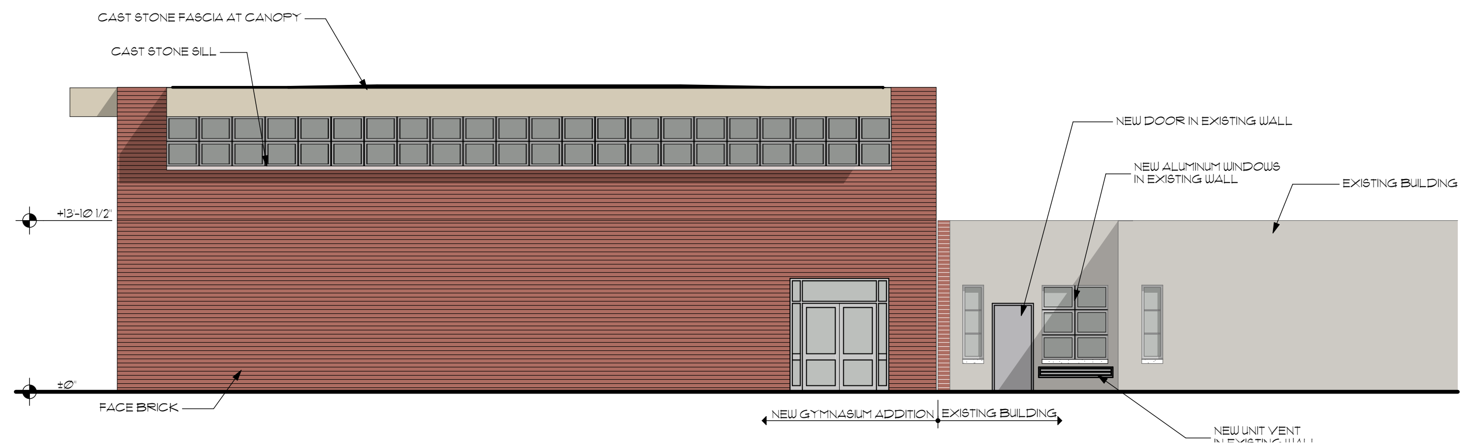
5 SOUTHEAST ELEVATION -- GYMNASIUM SCALE: 1/8" = 1'-0"
