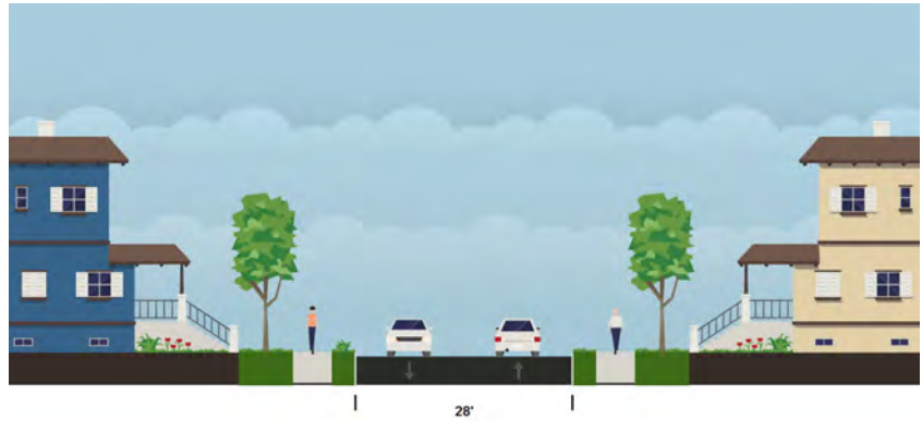
Figure 4.47 (a) - Existing Cross-section: Oakton Street
