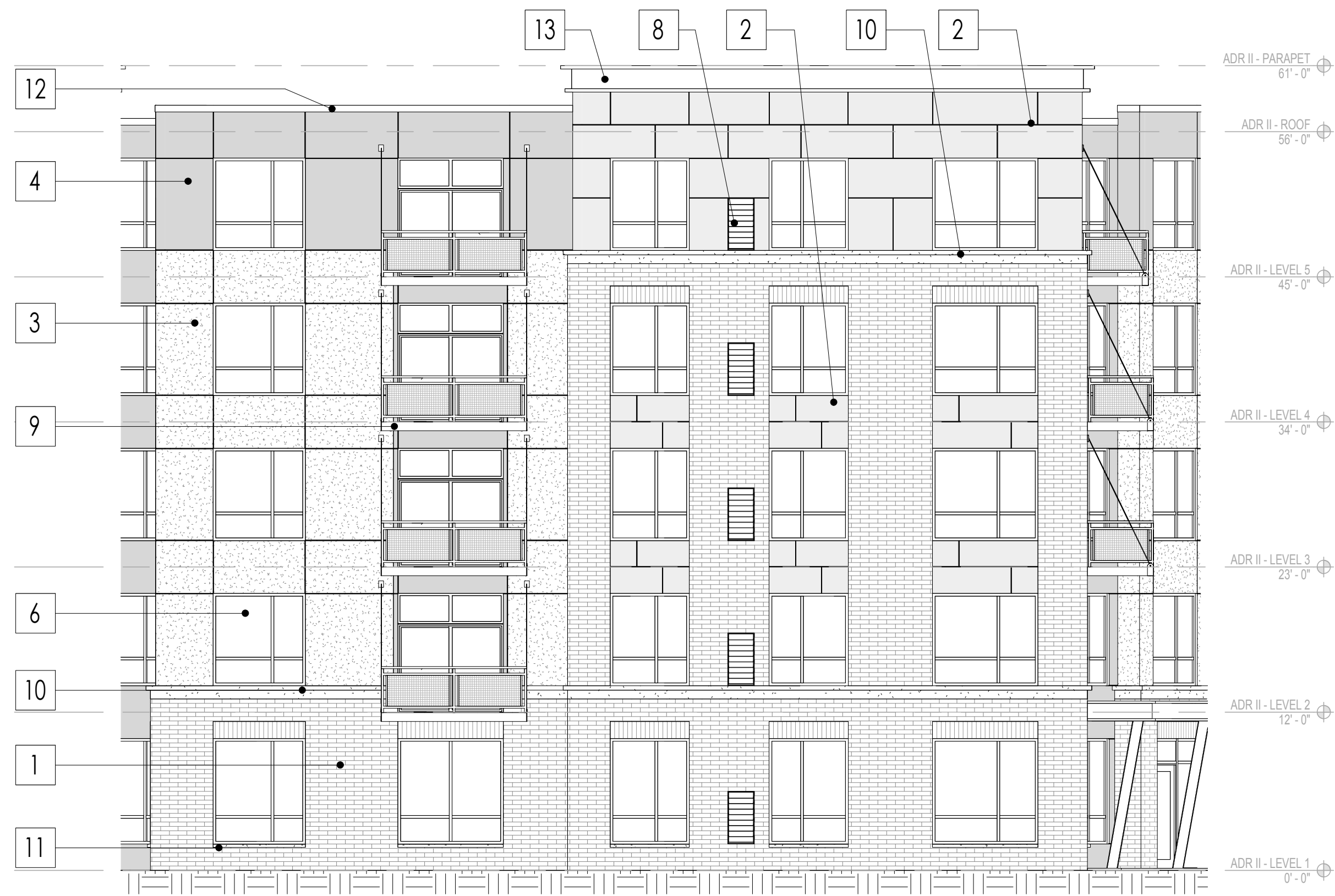
1 NORTHWEST ENTRY ELEVATION - DC SCALE: 1/8" = 1'-0"
