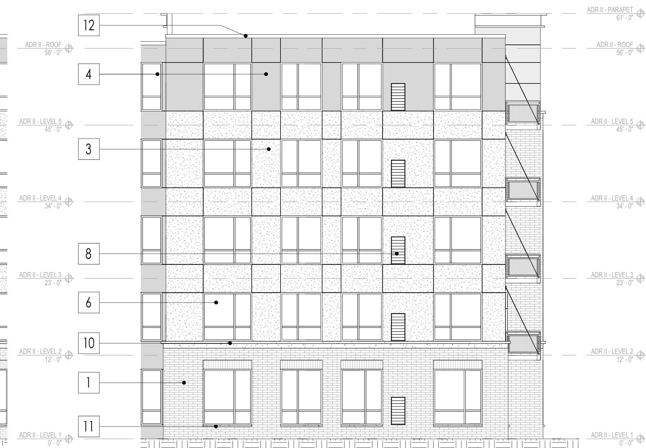
4 NORTHEAST ENTRY ELEVATION - DC SCALE: 1/8" = 1'-0"
