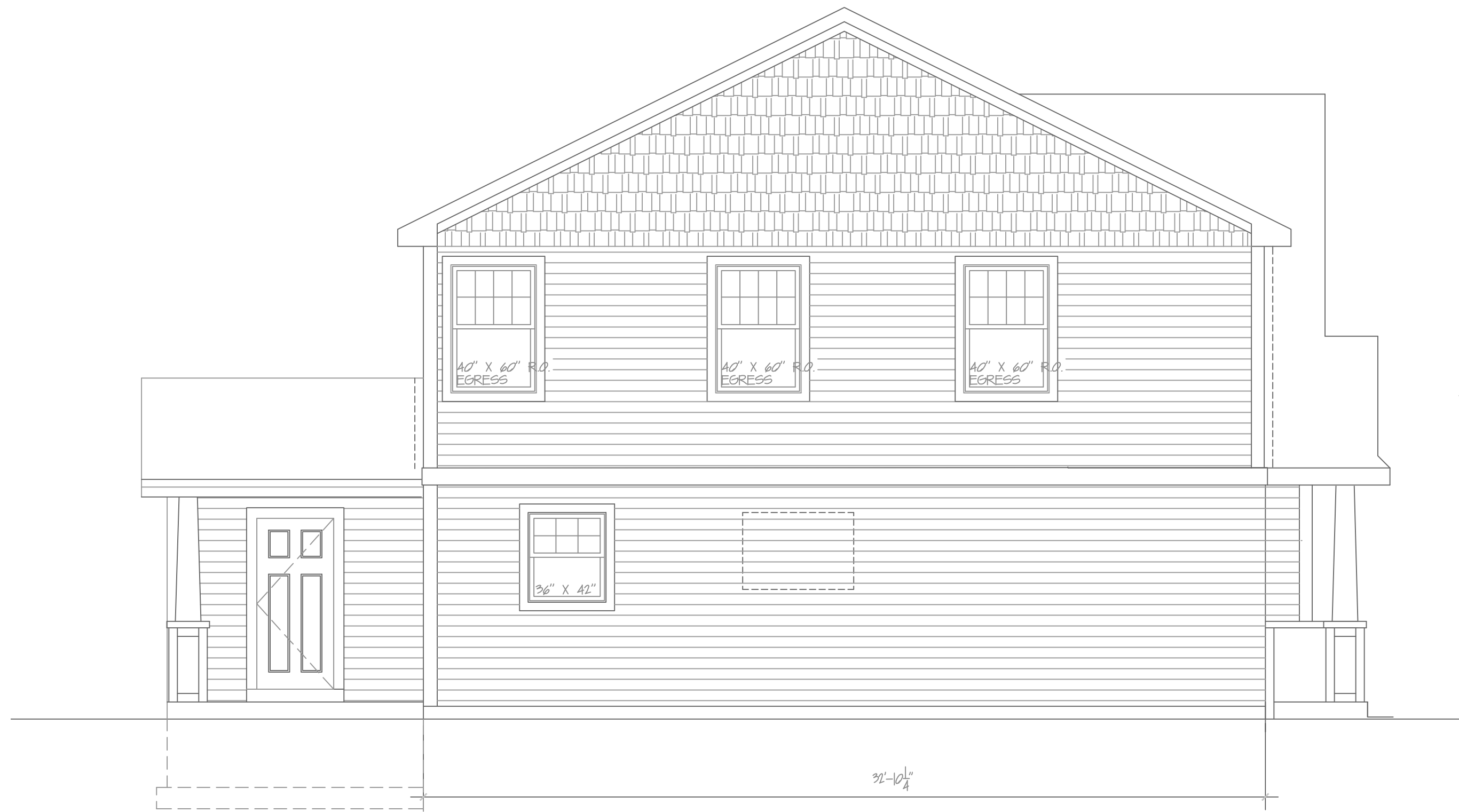
2 A3 PROPOSED LEFT (SOUTH) ELEVATION 1/4" = 1'-0"
