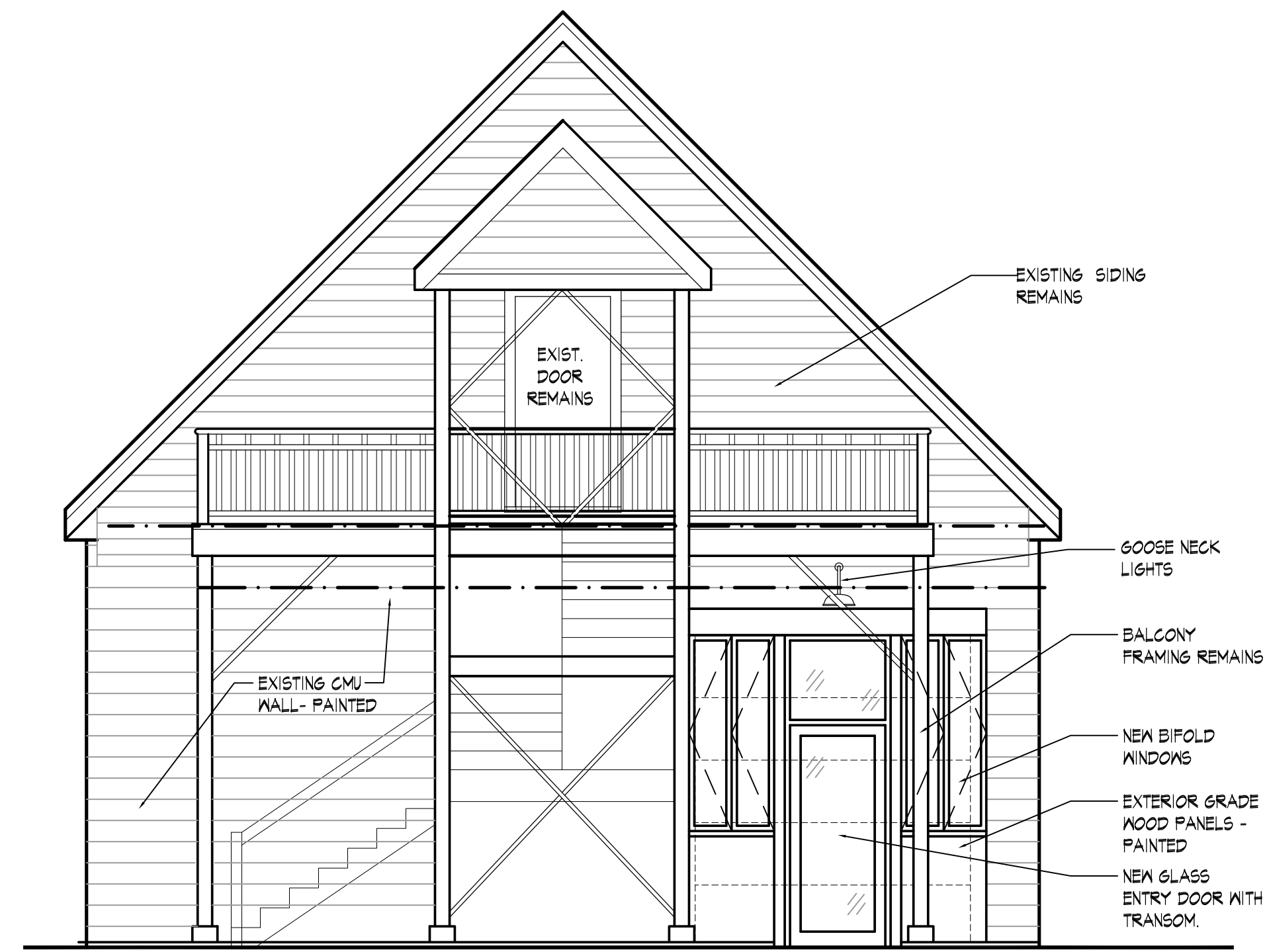
DEMO AND PROPOSED EXISTING BACK ELEVATION SCALE: 1/4" = 1'-0"
