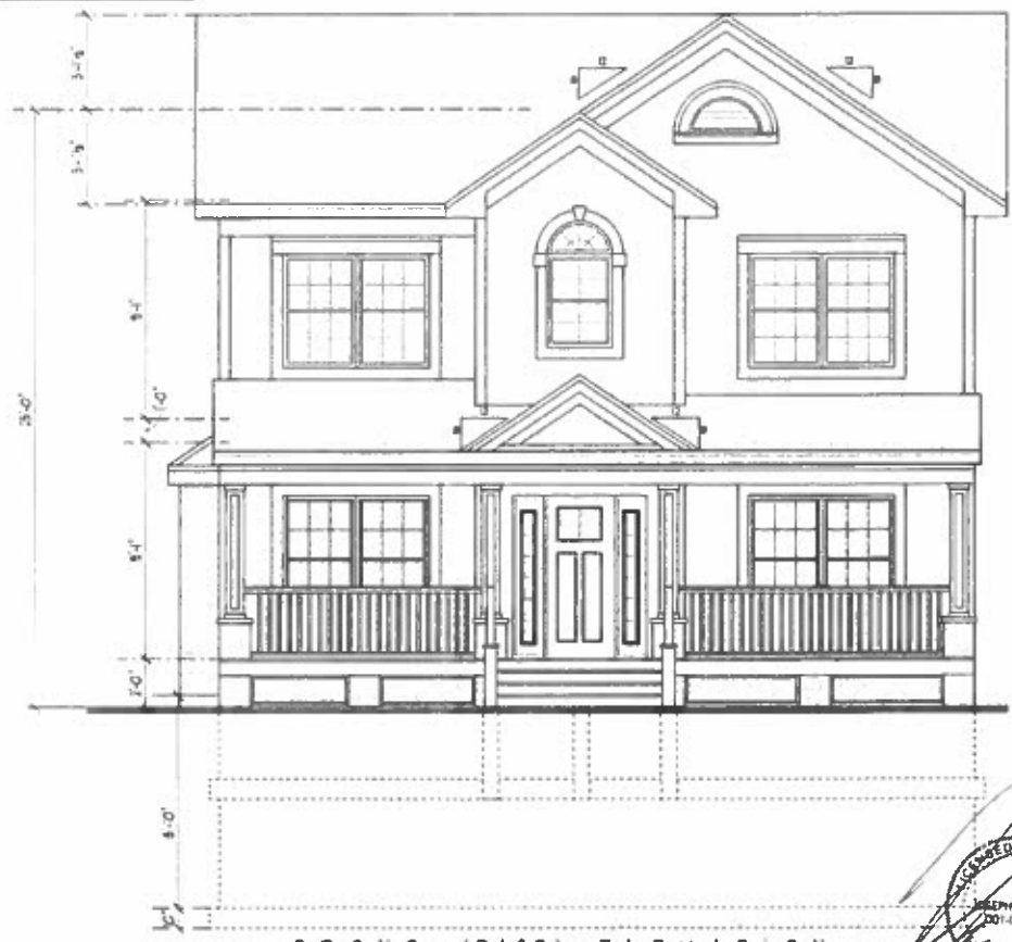
FRONT (EAST) ELEVATION (1/4" = 1'-0")
