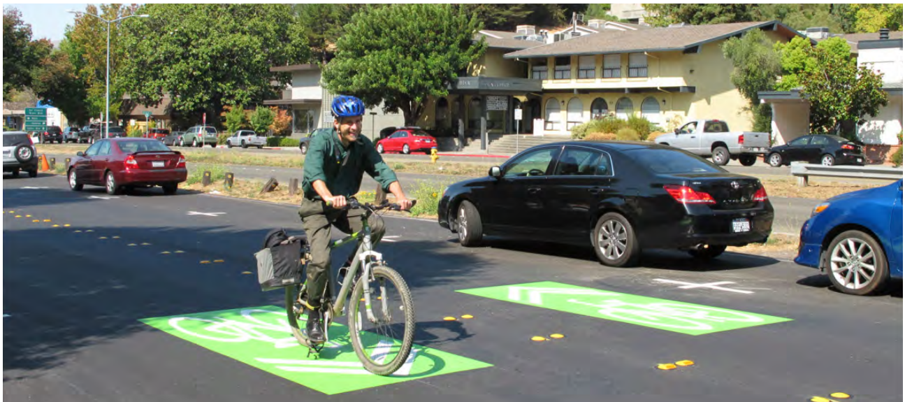
Figure 4.64 - High-visibility, green-backed sharrows (currently experimental)
