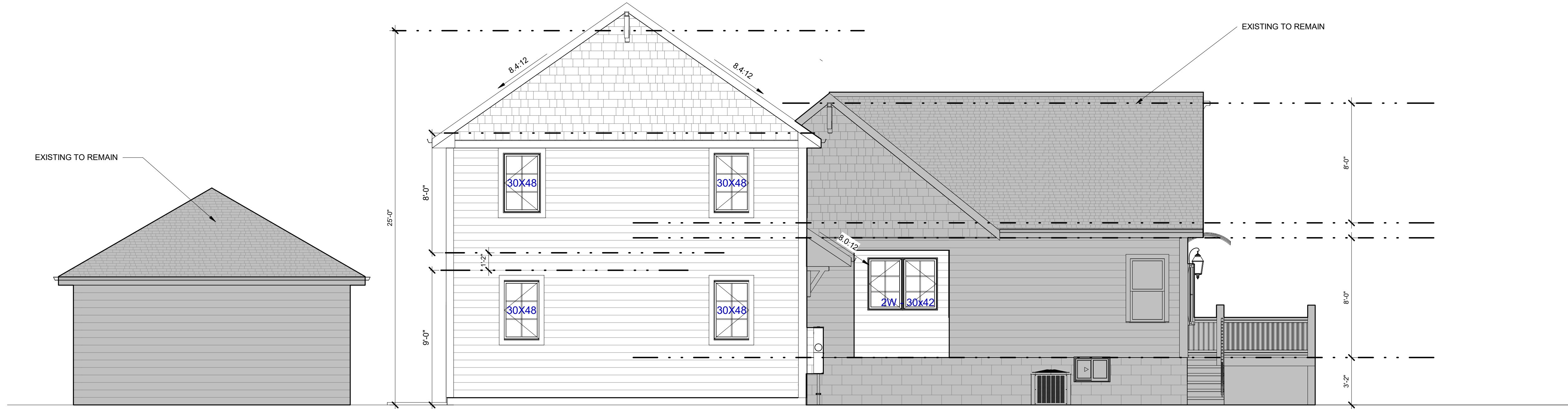
2 EAST ELEVATION - SIDE A3.0 1/4" = 1'-0"
