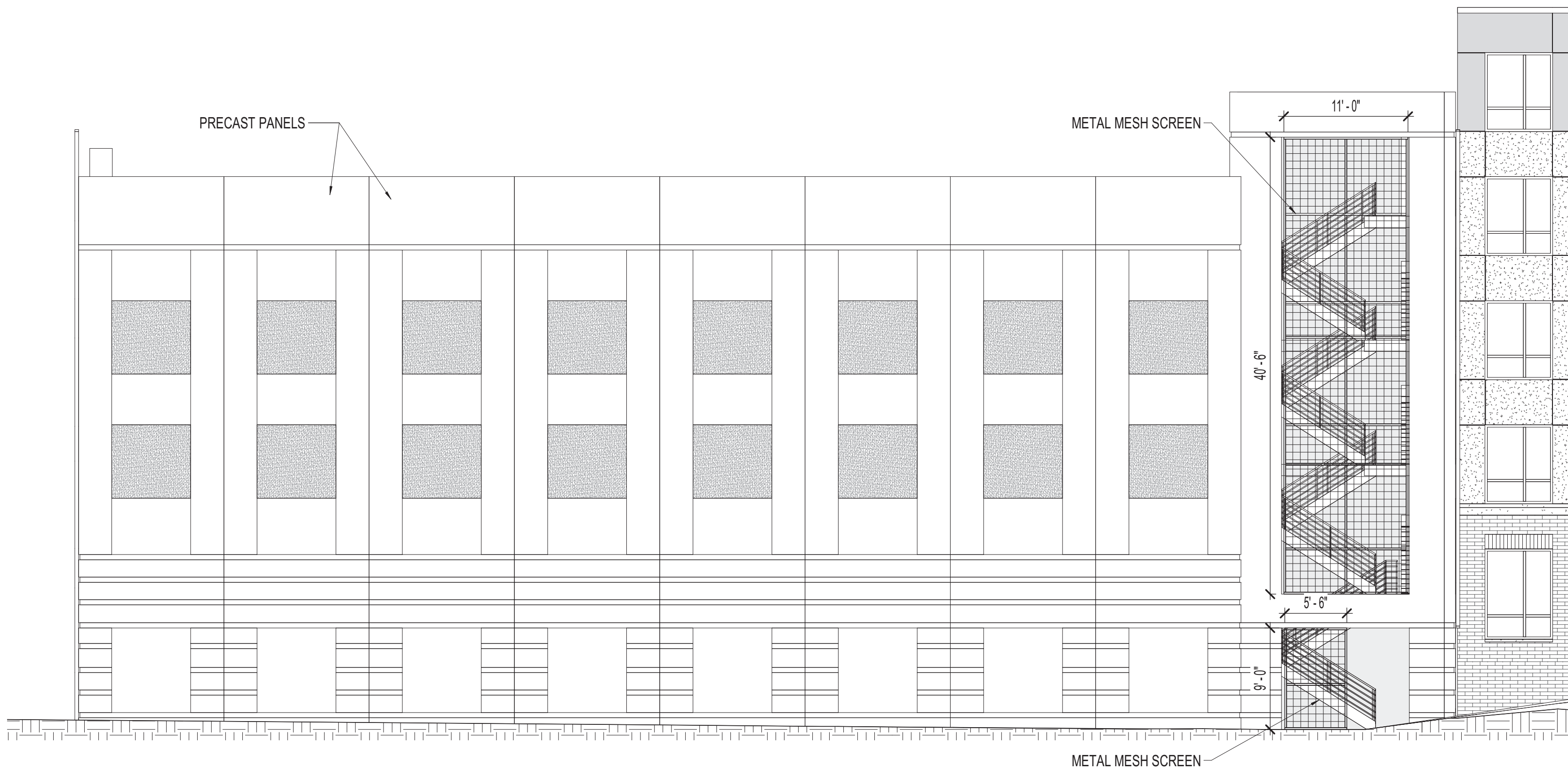
2 NORTH ELEVATION @ GARAGE - DC A206 SCALE: 1/8" = 1'-0"
