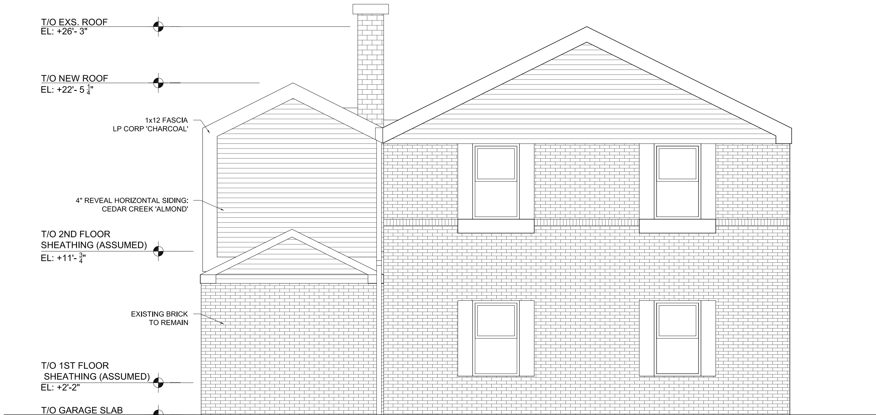
2 PROPOSED NORTH ELEVATION Scale: 1/4" = 1'
