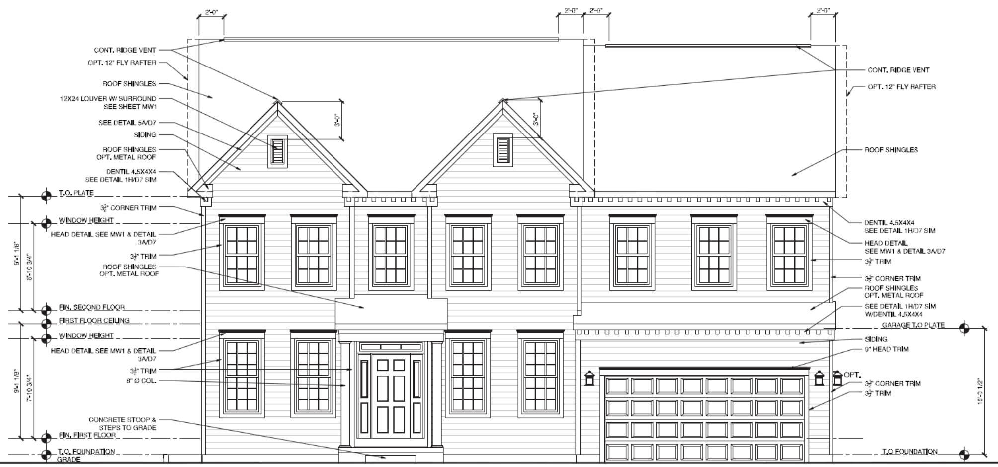
1 FRONT ELEVATION - FORM 'GS' (SIDING) SCALE: 1/4"=1'-0"
