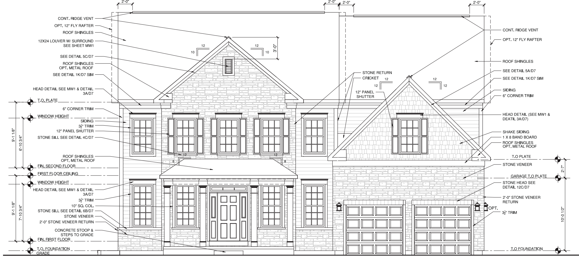
1 FRONT ELEVATION - FORM 'HT' (STONE) SCALE: 1/4"=1'-0"
