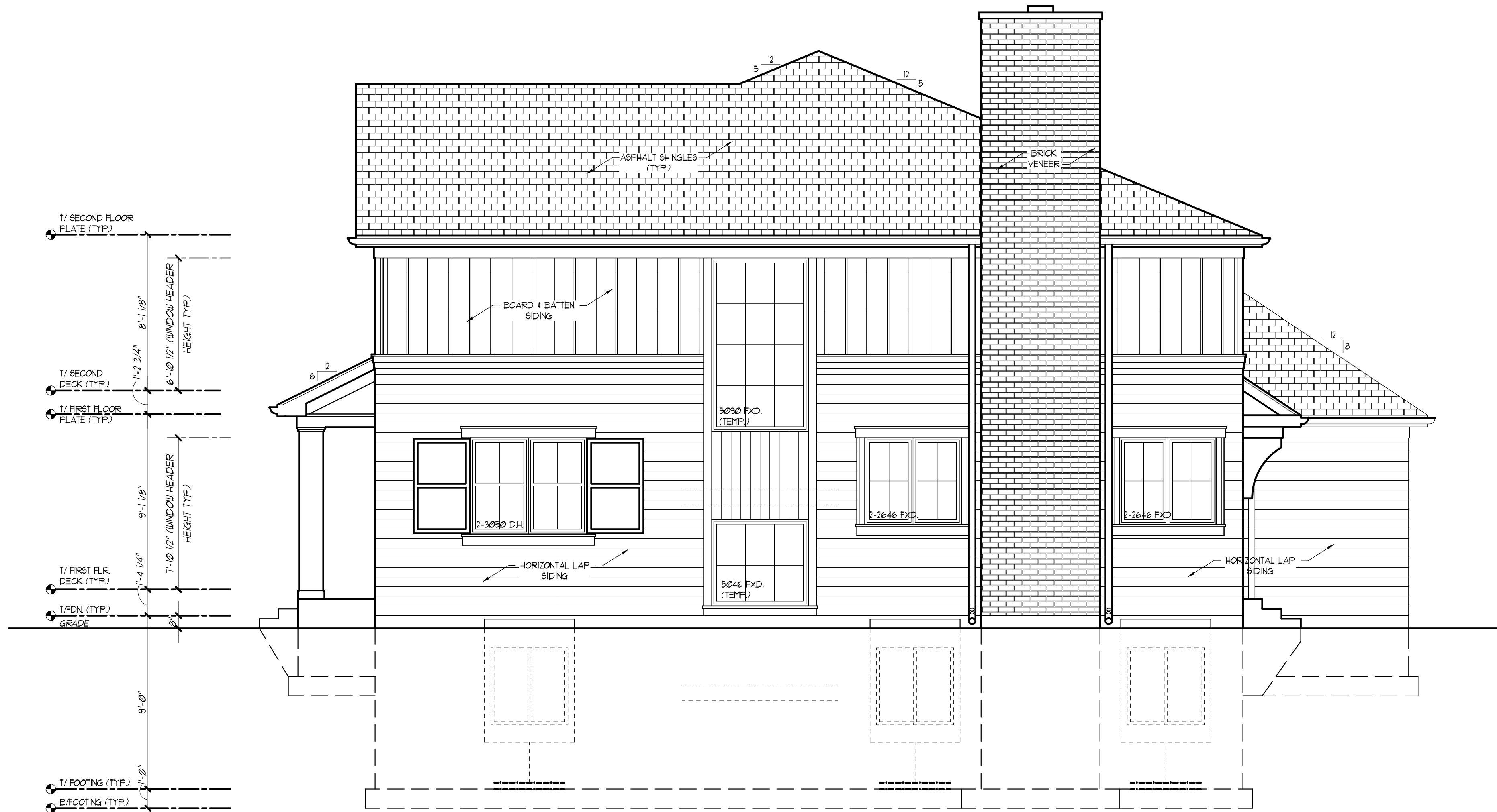
RIGHT SIDE ELEVATION SCALE: 1/4"=1'-0" JMB ARCHITECTS LTD.
