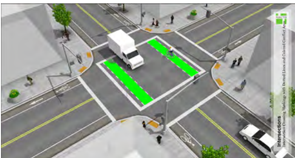
Continuous, solid colored pavement, outlined with the dashed white lines (or “elephant’s feet”)
