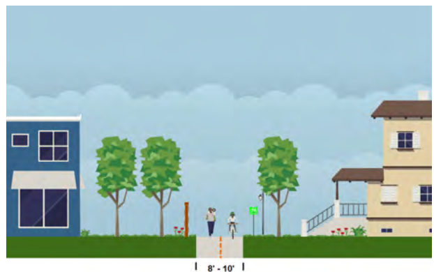
Figure 4.8 (b) - Proposed Cross-section: Cut-through Bikeway
