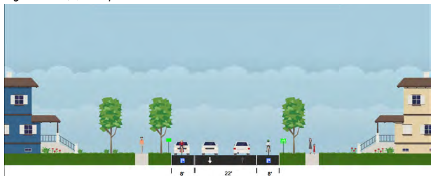
Figure 4.67 (b) - Proposed Cross-section: Burr Oak Street
