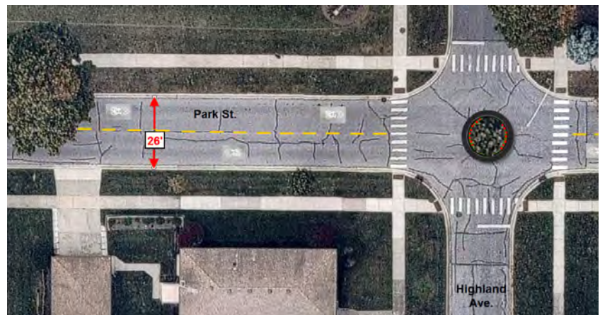
Figure 4.63 - Proposed Cross-section: Park Street at Highland Avenue Sharrows and Traffic Calming Concept
