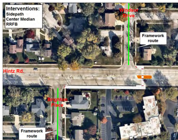
Hintz at Brighton-Windsor - Sidepath on south side, with raised center median (Note: See Appendix H for illustration of alternate design concept, with sidepath along north side of Hintz).
