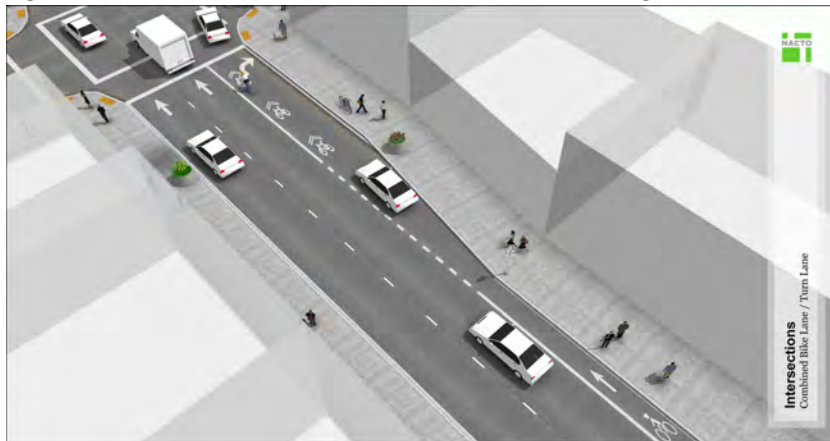
Figure 4.78 - Intersection Treatments: Combined Bike Lane / Right-Turn Lane
