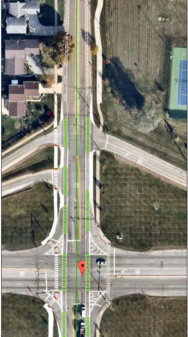
Figure 4.21 - Buffered bike lanes at Kennicott and Palatine
