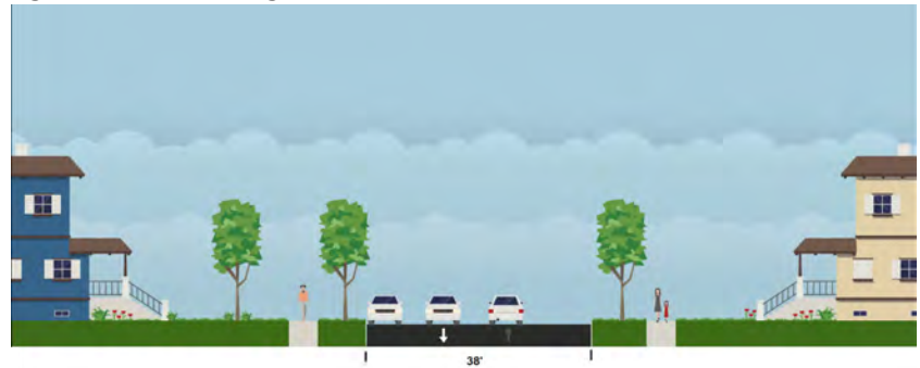
Figure 4.67 (a) - Existing Cross-section: Burr Oak Street
