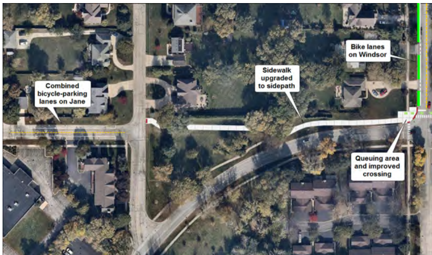
Figure 4.24 - Propose bikeway connection at Dryden and Windsor
