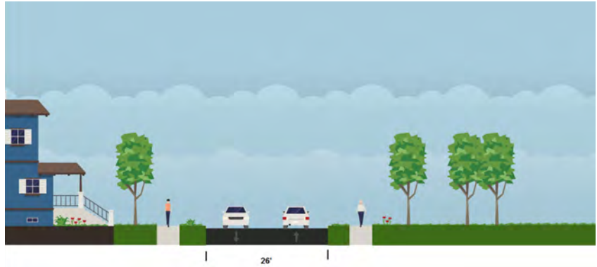
Figure 4.62 - Existing Cross-section: Park Street (26 ft.)
