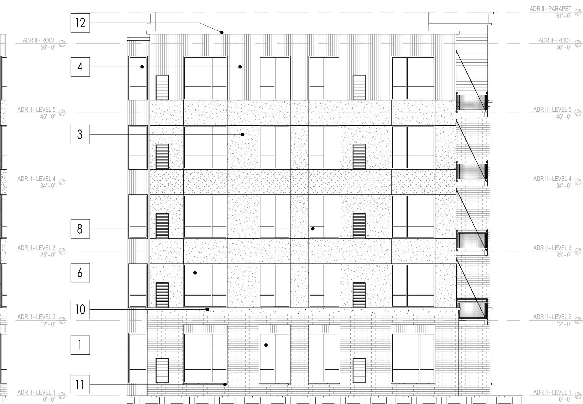
4 NORTHEAST ENTRY ELEVATION - DC SCALE: 1/8" = 1'-0"
