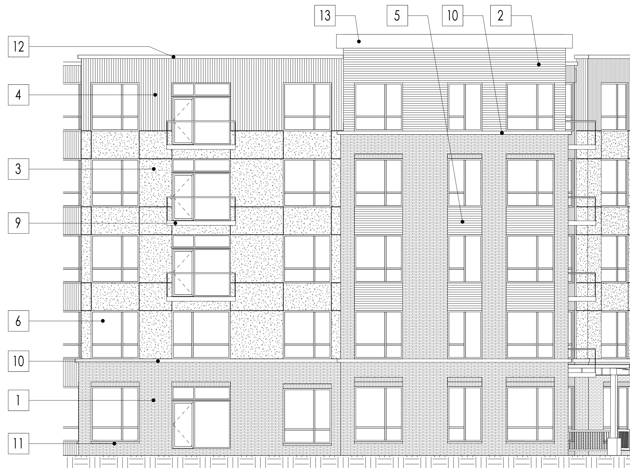
1 NORTHWEST ENTRY ELEVATION - DC SCALE: 1/8" = 1'-0"
