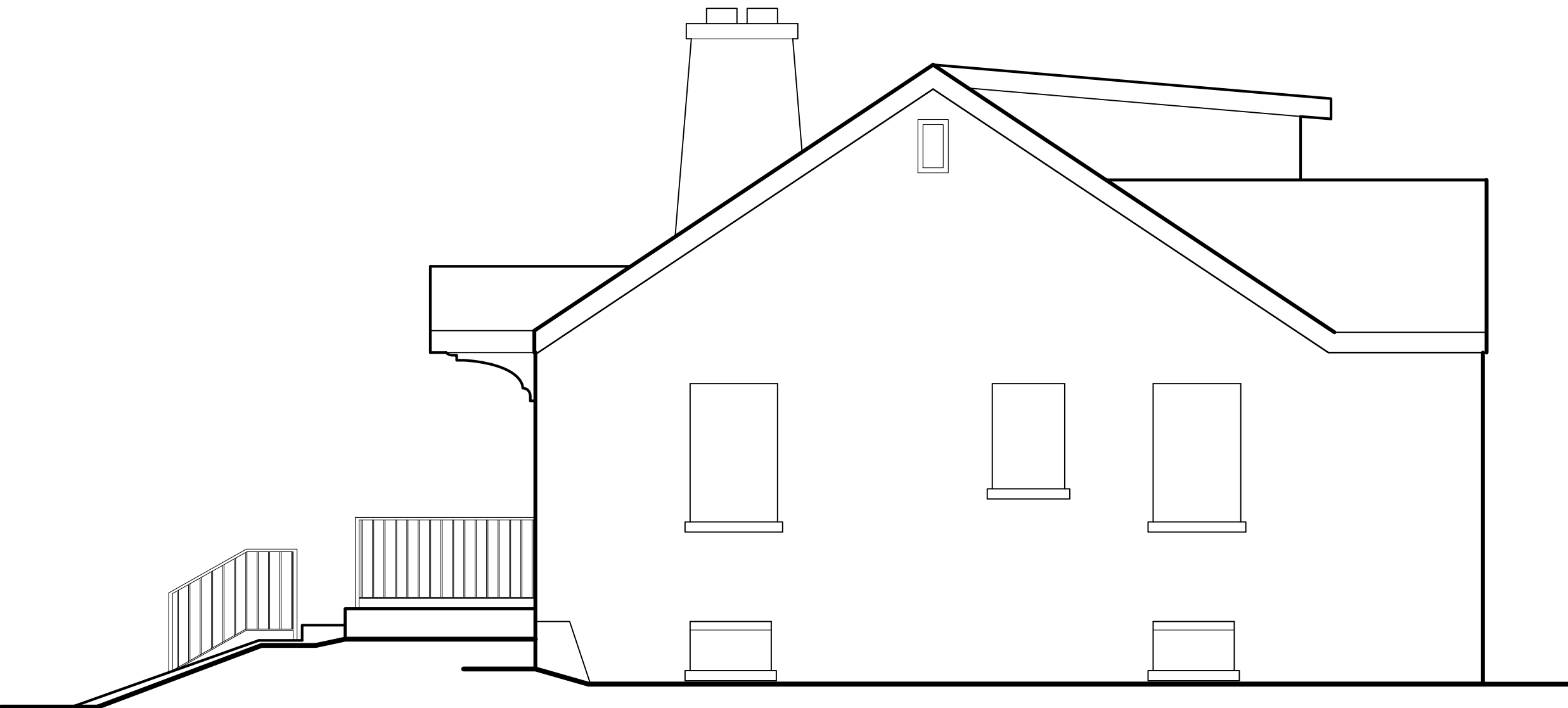
4 EXISTING SOUTH ELEVATION EX-2 1/4" = 1'-0"
