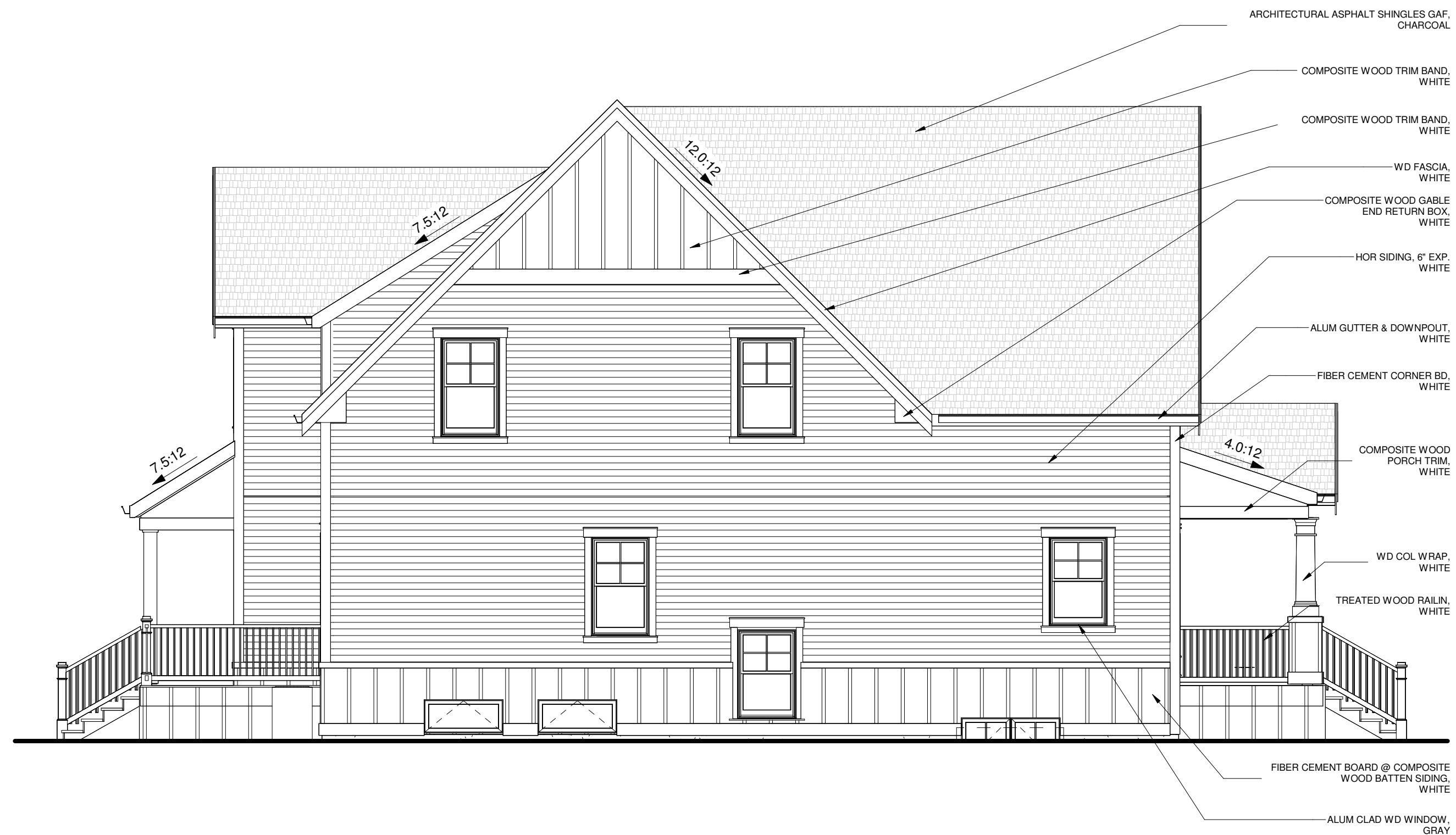
⑤ SIDE (NORTH) ELEVATION DC 3/16" = 1'-0"
