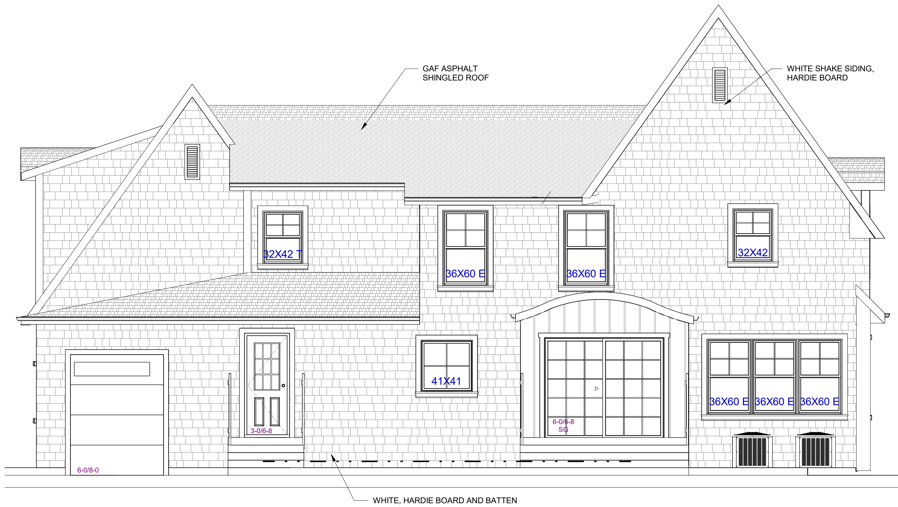
3 NORTH ELEVATION - REAR A6 1/4" = 1'-0"
