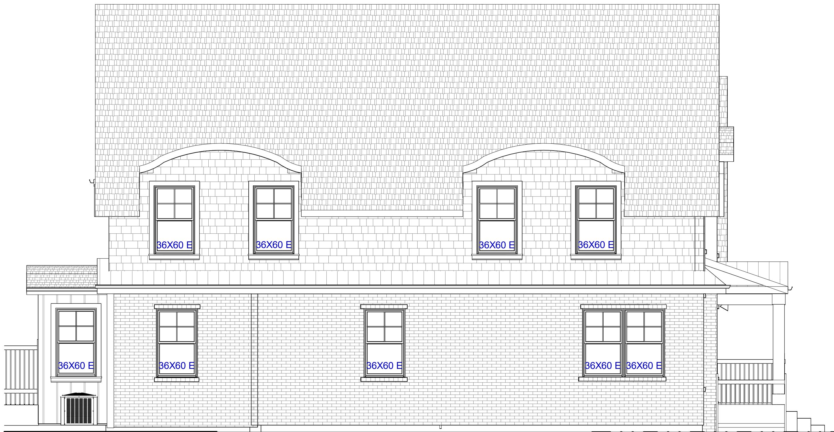
2 EAST ELEVATION - SIDE A6 1/4" = 1'-0"
