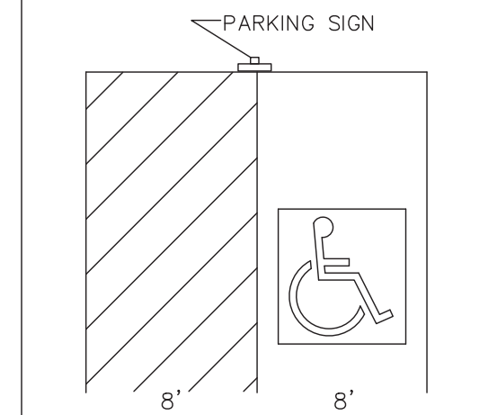
R7-8 ACCESSIBLE PARKING STALL N.T.S.
