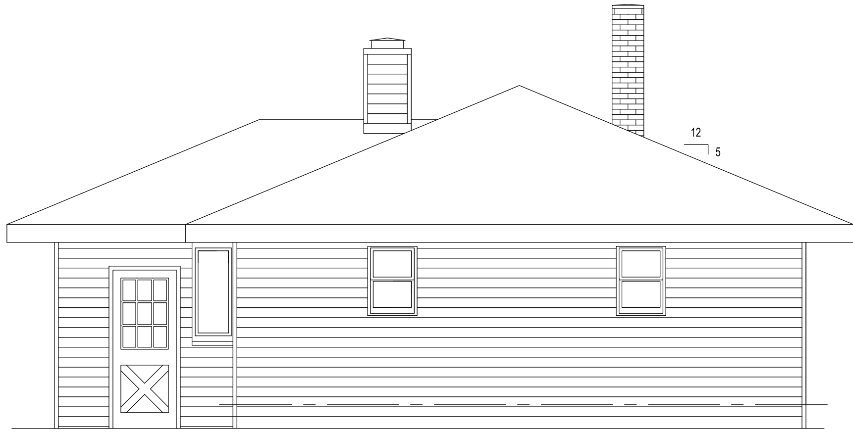
EXISTING WEST ELEVATION 1/4"=1'-0"
