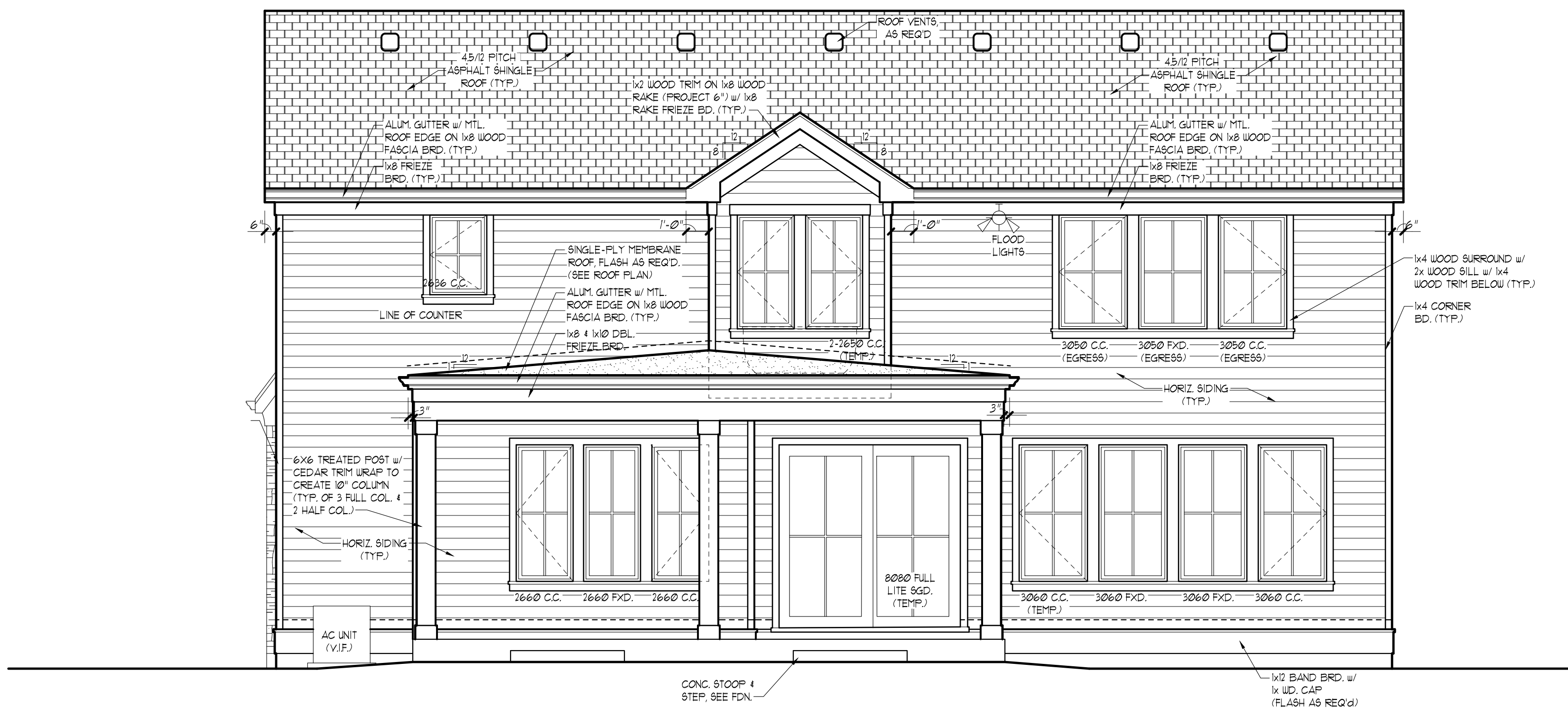
REAR ELEVATION SCALE: 1/4" = 1'-0" JMB ARCHITECTS LTD.
