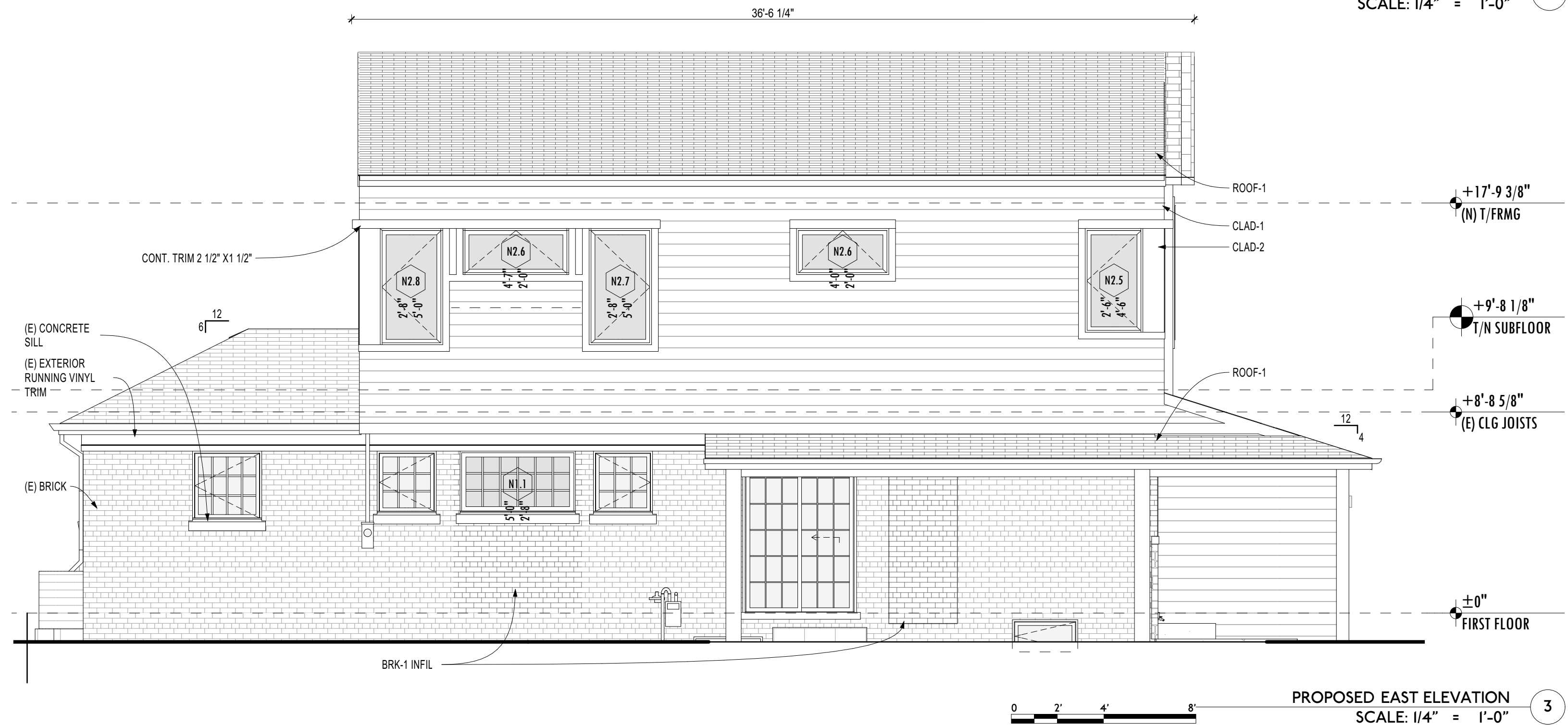
PROPOSED EAST ELEVATION - PORCH SCALE: 1/4" = 1'-0" (5)
