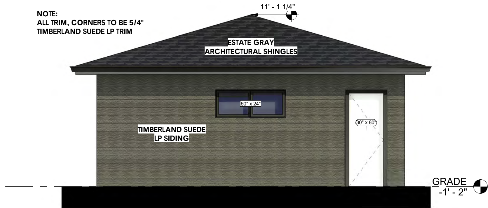
③ ELEVATION - GARAGE - WEST 1/4" = 1'-0"
