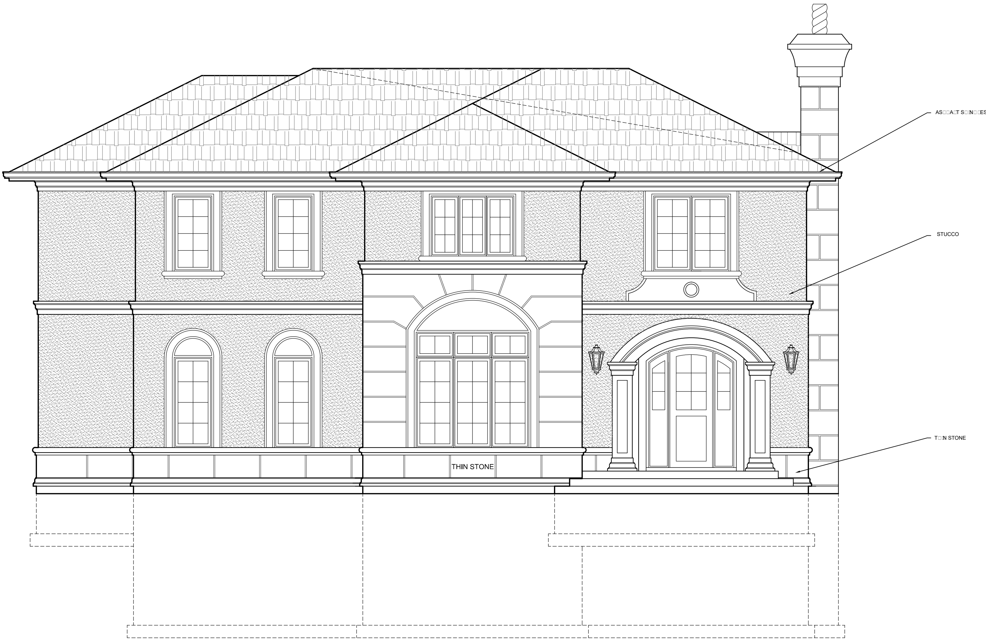
1 SOUTH ELEVATION FRONT BURBOYNE AVE SCALE 1/8"=1'-0"
