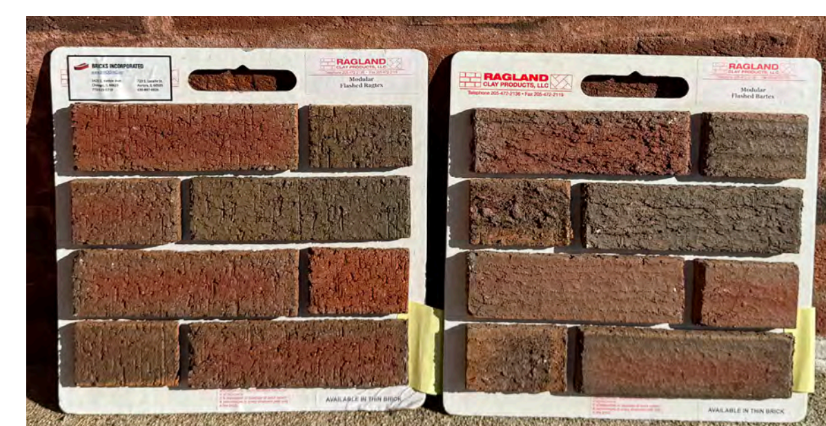
PROPOSED BRICK BLEND 80% FLASHED RAGTEX AND 20% FLASHED BARTEX (TO MATCH EXISTING)
