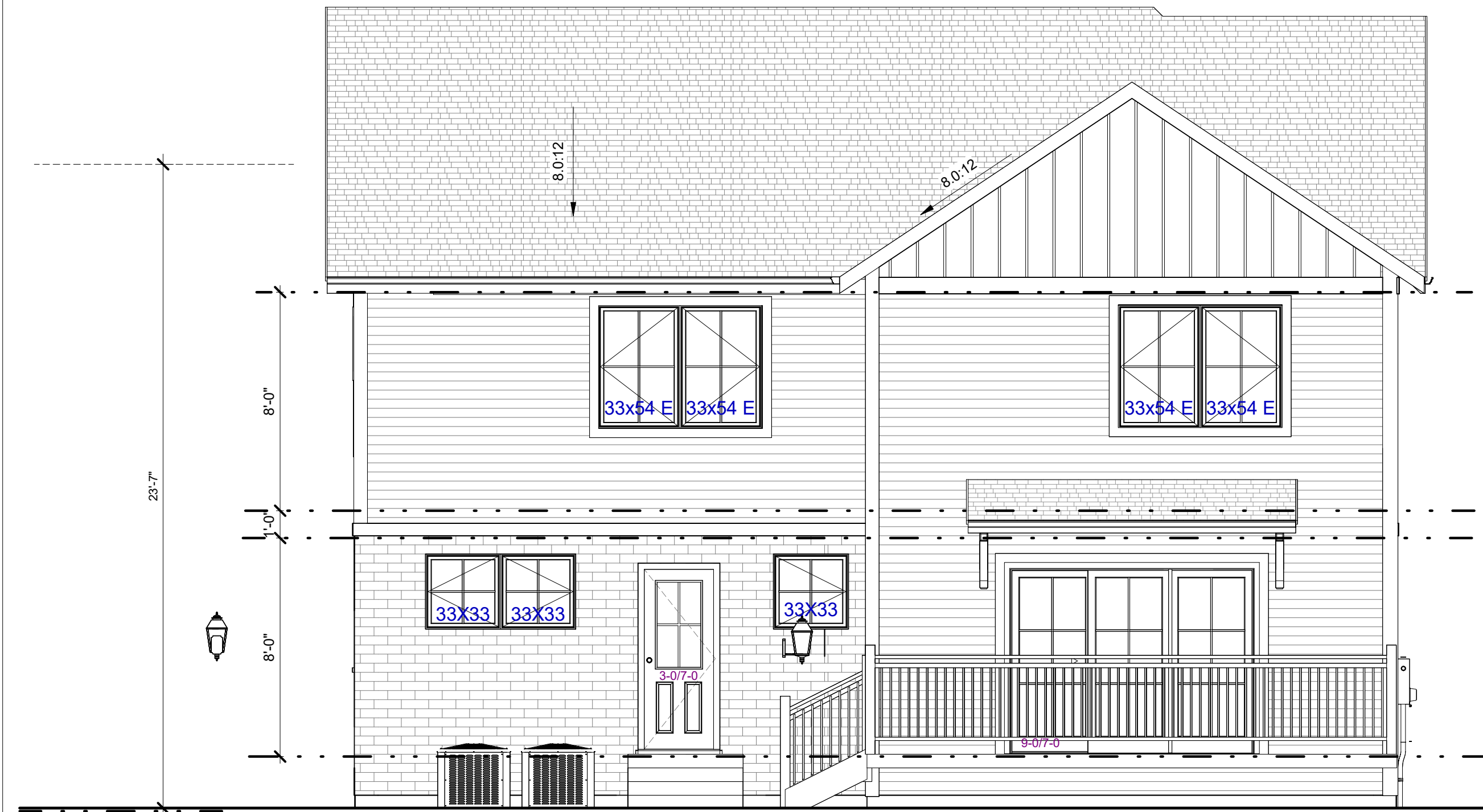
3 EAST ELEVATION - PROPOSED REAR A6 1/4" = 1'-0"
